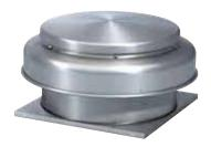
Designed for either supply or exhaust applications on natural gravity or positive pressure systems. Often used in conjunction with other HVAC products requiring an intake or exhaust vent. These units are low profile and have a rigid aluminum, corrosion resistant design providing a strong, long lasting, efficient and economical product. Integral birdscreen prevents entry of birds and other small objects. Built in curb cap with prepunched holes for easy attachment to roof curbs.
