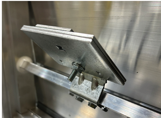
Figure 4: Bending counterbalance to reduce angle
