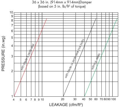
Leakage 36 x 36 in. (914mm x 914mm)Damper
