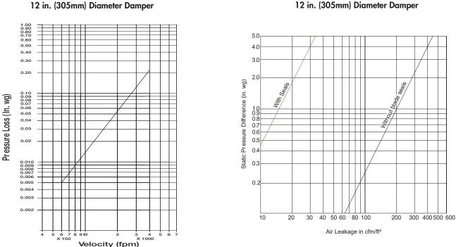
Leakage 12 in. (305mm) Diameter Damper
