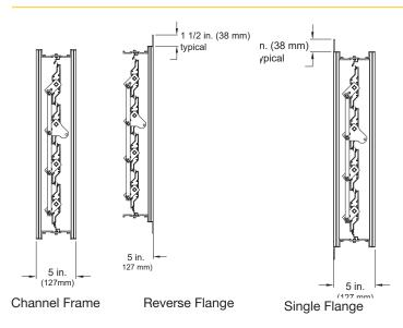
$^{\star}$  Width and height is based on outside dimension. W & H dimensions furnished approximately  $\frac{1}{4}$  in. (6mm) undersize.
