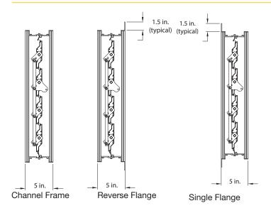
$^{\star}$  Width and height is based on outside dimension. W & H dimensions furnished approximately  $\frac{1}{4}$  in. (6mm) undersize.
