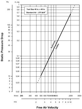
Model VAVH-5 resistance to airflow (pressure drop) varies depending on louver application (air intake or air exhaust). Free area velocities (shown) are higher than average velocity through the overall louver size. See louver selection information. (Test Figure 5.5)
