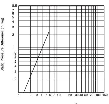
Air Leakage (cfm/ft<sup>2</sup>)
